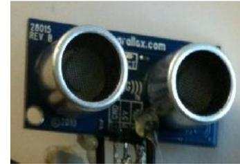
Figure 3: Parallax Ultrasonic Transducer
