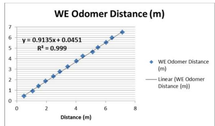
**Figure 8:** Wheel Encoder Distance Linear Interpolation
