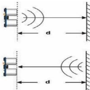
**Figure 9:** Ultrasonic Sensor Operation [5]
