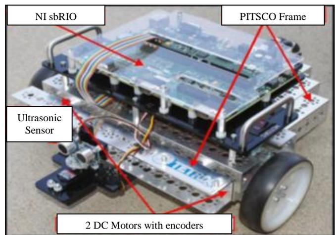
Figure 1: DANI Robot (Robotic Starter Kit1) [9]
