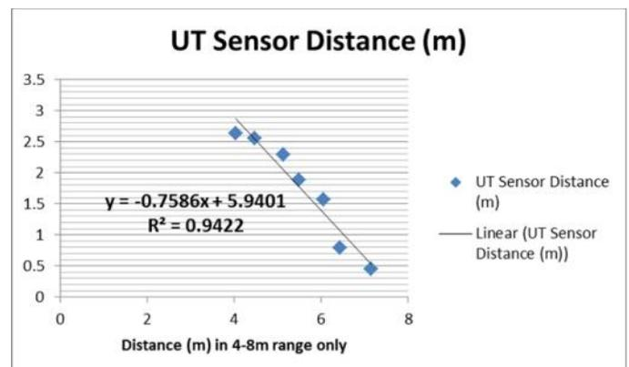
**Figure 11:** Ultrasonic Sensor Distance Linear Interpolation (within 4m of reflecting wall, only)
