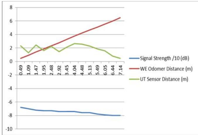
Figure 6: Three Localization Method Results Vs. Distance travelled by Robot
