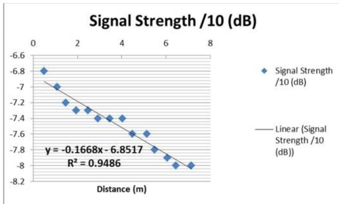
Figure 12: Received Signal Strength Linear Interpolation
