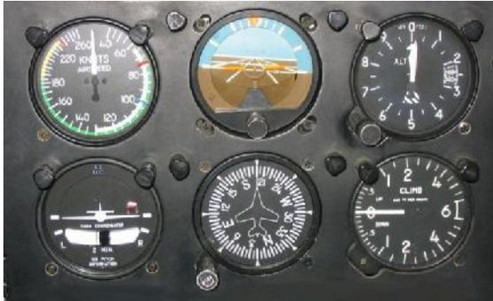
Figure 12. Six primary flight instruments
