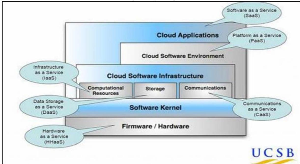
**Figure 4:** Different layers of cloud computing [9]
