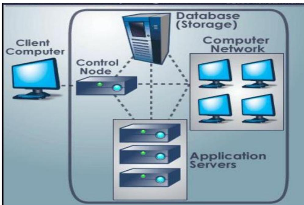
**Figure 3:** Typical structure of cloud computing system [7]
