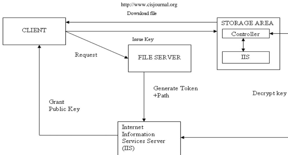
**Figure 9:** SSL control flow diagram
